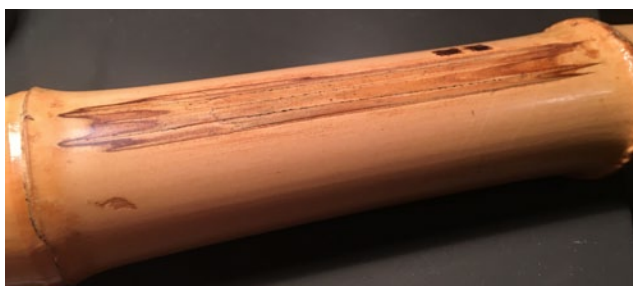
Mark resulting from constant rubbing of two culms
