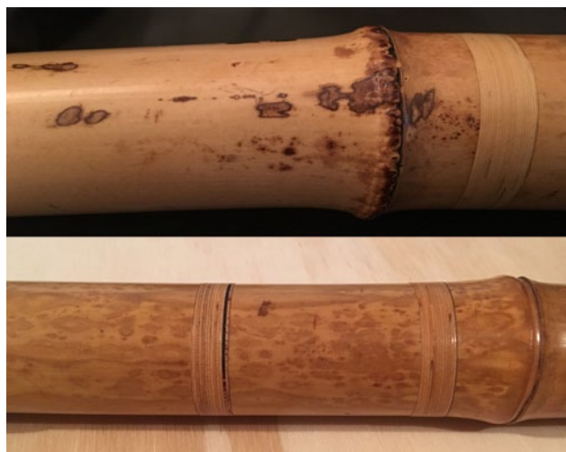
Mottling caused by fungus
